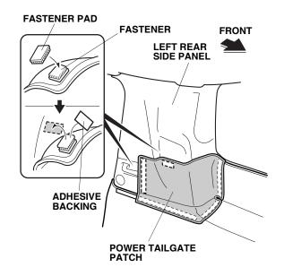
25. Remove the adhesive backing from two fastener pads, fold the power tailgate patch over, and attach the two fastener pads to the left rear side panel. Press the two fastener pads firmly against the side panel with the rubber roller. Go to step 30.
