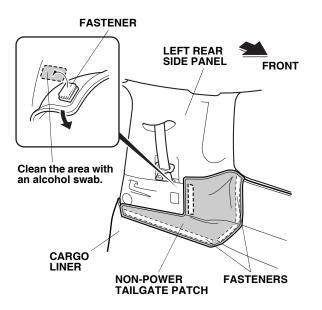
27. Align the non-power tailgate patch to the left rear side panel, fold the non-power tailgate patch over and, using an alcohol swab, thoroughly clean the area where the fasteners will attach. After cleaning with the alcohol swab, wait at least 3 minutes before continuing with the next step.
