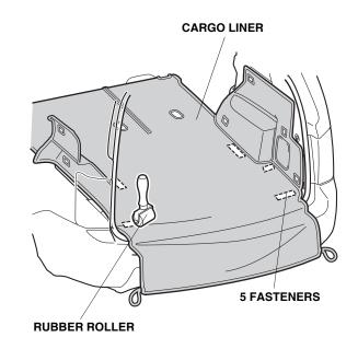
8. Align the cargo liner to the right rear side panel, fold the cargo liner over and, using two alcohol swabs, thoroughly clean the area where the fasteners will attach. After cleaning with the alcohol swabs, wait at least 3 minutes before continuing to the next step.
