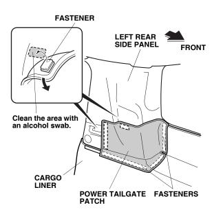
23. Align the power tailgate patch to the left rear side panel, fold the power tailgate patch over and, using an alcohol swab, thoroughly clean the area where the fasteners will attach. After cleaning with the alcohol swabs, wait at least 3 minutes before continuing with the next step. 24. Locate the two fasteners on the power tailgate patch and attach two fastener pads to the power tailgate patch as shown.
