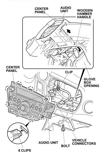
With Navigation: Insert your hand through the glove box opening, and push the back of the navigation unit forward to release the seven clips. Release the harness clip, and unplug the vehicle connectors. Carefully remove the navigation unit without scratching the dashboard.
