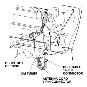
45. If necessary, reposition the excess antenna cord, and tighten the wire tie loosely installed in step 23.
