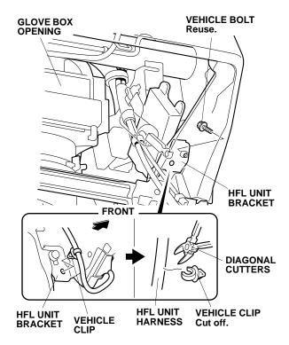
35. Remove the vehicle bolt from the HFL unit bracket.
