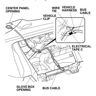
27. Secure the bus cable to the vehicle harness at electrical tape C with one wire tie.
