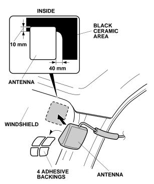
15. Remove four adhesive backings from the antenna, and attach the antenna to the windshield as shown. Firmly press the antenna against the windshield to ensure good adhesion.
