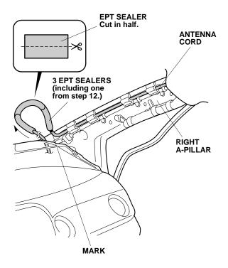
23. Route the antenna cord down to the glove box opening. Loosely secure the excess antenna cord to the vehicle harness with one wire tie.
