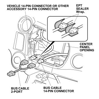
48. Plug the bus cable 14-pin connector into the audio-navigation unit or the audio unit, reconnect the other vehicle connectors, and reinstall the center panel.
