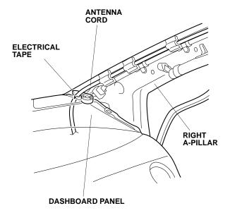
22. Using scissors, cut one EPT sealer in half. Wrap these pieces, plus the piece you cut in step 12, around the antenna cord, starting from the tape mark you made in step 21 and working downward.
