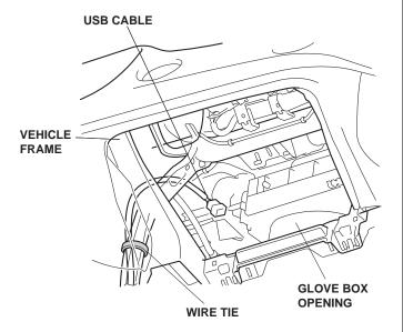
30. Secure the USB cable to the vehicle harness with one wire tie.
