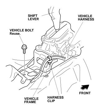
14. Position the control unit bracket under the floor carpet as shown.
