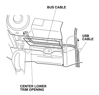
26. Align the bus cable 14-pin connector with the vehicle 24-pin connector, and secure the bus cable to the vehicle harness with one wire tie.
