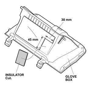
32. Using a pushpin, pierce the glove box in two places at the measurements shown.
