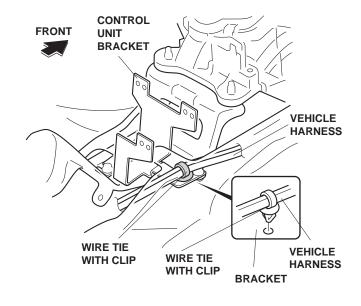
18. Install the control unit to the control unit bracket with three 5 x 7 mm flange bolts. Use a combination wrench to tighten the flange bolts.
