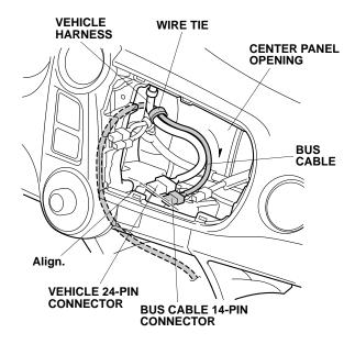
27. Bundle the excess bus cable, and secure it to the vehicle frame with two wire ties.
