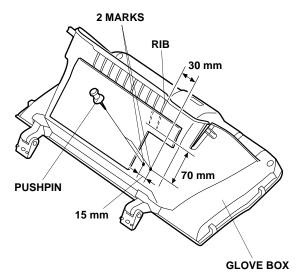
33. While wearing eye protection, drill the two pierced marks in the glove box. First drill with a 3 mm drill bit, and finish with a 16 mm hole saw. Use a utility knife to cut between the two 16 mm holes. Remove any burrs.
