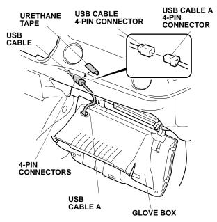
37. Wrap one urethane tape around the 4-pin connectors.
