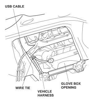
31. Get the glove box. Using a utility knife, cut out the insulator on the glove box at the measurement shown.
