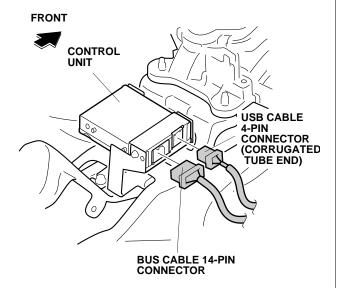
20. Route the bus cable and the USB cable forward along the vehicle harness.
