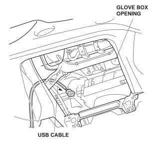
29. Secure the USB cable to the vehicle frame with one wire tie.
