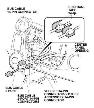
41. Plug the bus cable 14-pin connector or bus cable 2-port 14-pin connector into the audio unit, and reinstall the audio unit.
