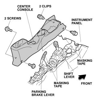
12. Carefully remove the center console (two clips and two screws).
