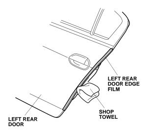
23. Repeat steps 1 through 22 to install the door edge film on the right side of the vehicle.
