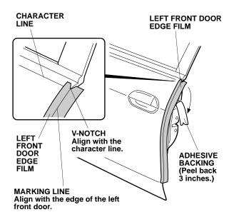
7. When the alignment is correct, apply light pressure to the door edge film while you carefully remove the adhesive backing. Don't worry about wrapping the door edge film around the door at this time. 8. Starting from the center and working outward, use the applicator with the soft sleeve to smooth out the left front door edge film. Move the applicator in only one direction.
