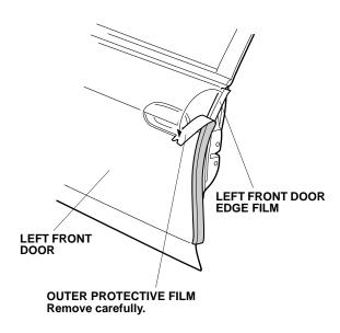
Starting from the center and working outward, fold the left front door edge film around the left front door edge. Be careful not to damage the door seal during this procedure.
