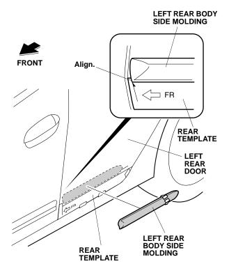
14. Press on the left rear body side molding firmly with the palm of your hand while removing the adhesive backings. Remove about 2 to 4 inches at a time.
