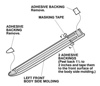
Align the left front body side molding with the front template, and attach it to the left front door. If the vehicle has door edge film installed, align the end with the door edge film.
