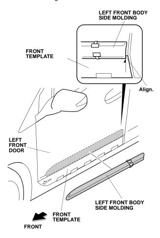
6. Press on the left front body side molding firmly with the palm of your hand while removing the adhesive backings. Remove about 2 to 4 inches at a time while pressing on the molding with the palm of your hand.
