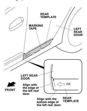
11. Place the left rear body side molding against the rear template to verify the installation position on the left rear door. Remove the body side molding.
