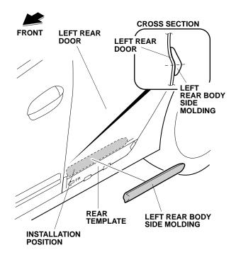
12. Peel back approximately 1½ to 2 inches of the adhesive backing from each adhesive tape, and tape the ends to the outside surface of the body side molding. Remove the small end pieces of the adhesive backing.
