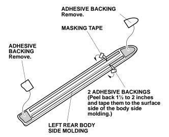
13. Align the left rear body side molding with the rear template, and attach it to the left rear door.
