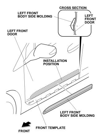
4. Peel back approximately 1½ to 2 inches of adhesive backing from each adhesive tape, and tape the ends to the front surface of the body side molding. Remove the small end pieces of the adhesive backing.
