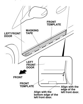
3. Place the left front body side molding against the template to verify the installation position on the left front door. Remove the body side molding.
