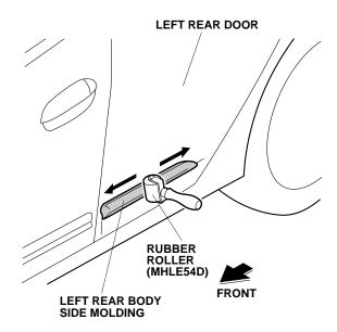
17. Turn the template over, and repeat steps 1 thru 16 to install the body side moldings on the right side of the vehicle.
