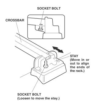
9. Install the roof racks with 12 socket bolts and 12 washers.
