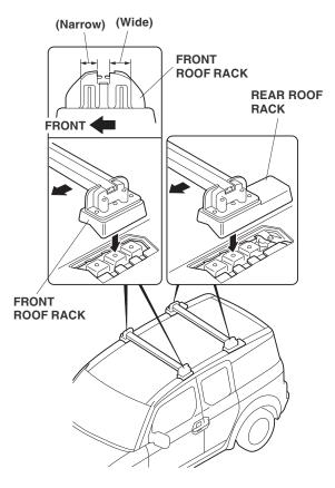
8. If the ends of the roof rack are not aligned, adjust them by loosening the crossbar socket bolts and moving the stays in or out as necessary.
