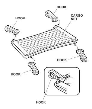
2. Attach the upper straps of the cargo net to the upper cargo area hooks as shown. Attach the cargo net hooks to the lower anchors in the cargo area as shown.
