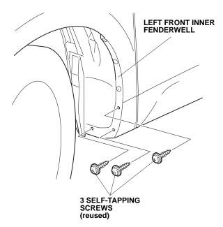
4. Secure the left front splash guard by tightening the three self-tapping screws (reused) and one 5 x 25 mm self-tapping screw (provided), in the order shown.
