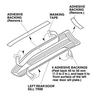
8. Starting at the curved area, bend the left rear door sill trim against the left rear door sill. Align the edge of the left rear door sill trim with the masking tape, and install the left rear door sill trim.
