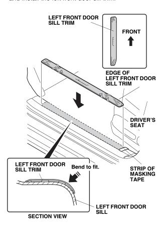
Using the palm of your hand, press the left front door sill trim firmly against the door sill, and remove the adhesive backing in the order shown. Apply firm pressure, especially at the ends.
