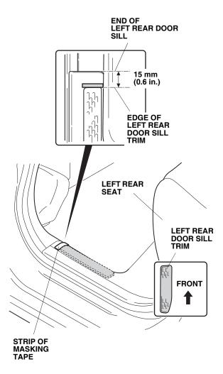
3. Using one alcohol wipe, clean the front and rear door sills where the door sill trims will attach. Allow the alcohol to dry.
