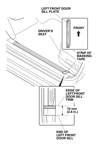
2. Open the left rear door. Place the door sill trim on the door sill at the measurement shown, and mark the door sill using a strip of masking tape at the edge of the door sill trim.
