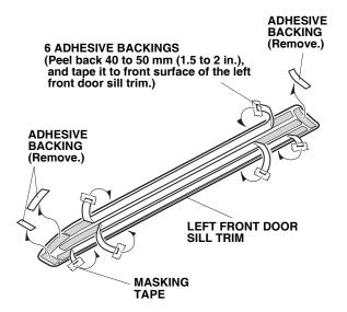
Starting at the curved area, bend the left front door sill trim against the left front door sill. Align the edge of the left front door sill trim with the masking tape, and install the left front door sill trim.
