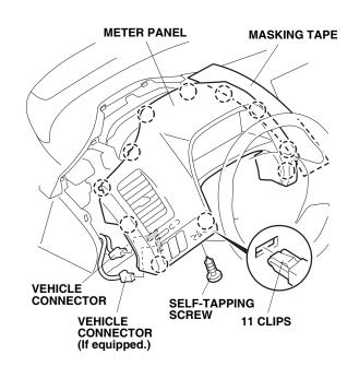
11. Apply masking tape to the instrument panel as shown. Remove the center panel (two bolts, 11 clips, an aspirator hose, and unplug the vehicle connectors).
