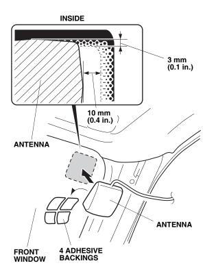
25. Remove the adhesive backings from the antenna, and attach the antenna to the location shown. Apply sufficient pressure to completely contact. 26. Attach masking tape to the location shown on the outside of the windshield.
