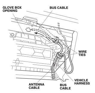
38. In the glove box opening, route the bus cable along the vehicle harness and towards the audio unit opening.
