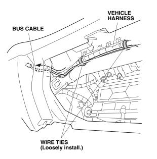
39. Using two wire ties, loosely install the bus cable to the vehicle harness.
