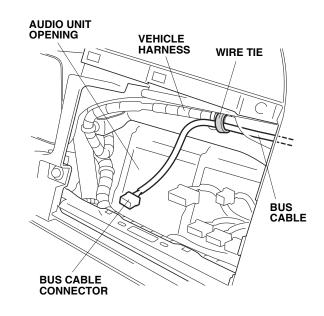
41. Bundle up the excess antenna cable as shown, and secure it with the two wire ties installed in step 39.
