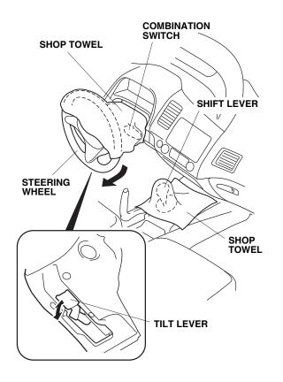
9. To protect the dashboard area, put shop towels over the steering wheel and shift lever.
