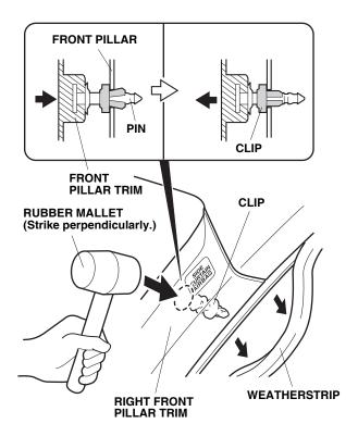
13. Push the clip into the vehicle side by striking the top of the right front pillar trim in the area marked "SIDE CURTAIN AIRBAG" with a rubber mallet perpendicularly to the pillar. Then, remove the clip. 14. Pull the weatherstrip off in the area shown. And remove the right front pillar trim (two clips).
