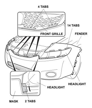
14. Pull the mask back toward the wheelwell, smooth out any wrinkles, and then snap the mask onto the snapscrew (A). Repeat on the other side.
