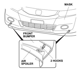
19. Route the elastic cord through the eight loops on the bottom of the mask. Attach one S-hook to the bottom edge of the bumper on one side. Stretch the cord, then attach the other S-hook to the bottom edge of the bumper on the other side.
