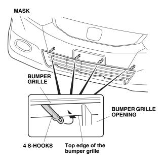
17. Attach the five S-hooks to the bottom inside edge of the bumper grille opening.
