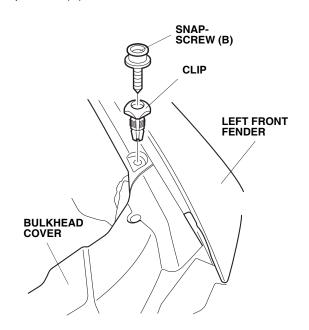
4. Repeat steps 2 and 3 to install a snap-screw (B) on the right side of the vehicle.
