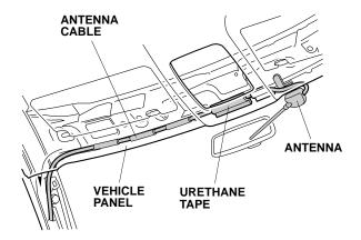
34. Route the antenna cable along the left A-pillar and secure it to the vehicle harness with five wire ties as shown.
