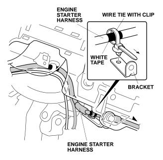
63. Route the engine starter harness 7-pin connectors (brown, green, white) to the steering column.
