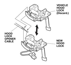
92. Attach the hood lock opener cable to the new hood lock.
