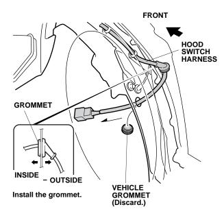
98. Route the hood switch harness along the vehicle harness to the center of the vehicle. Secure the hood switch harness to the vehicle harness with six wire ties.
