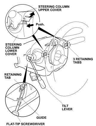
20. Remove the steering column upper cover (three retaining tabs).
