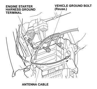
48. Remove the vehicle ground bolt from the vehicle. Secure the engine starter harness ground terminal with the vehicle ground bolt.
