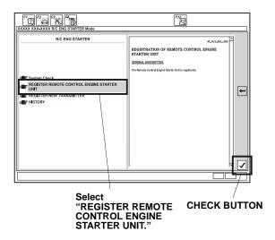
Check that "Obtain PCM-code (IMMOBILIZER PCM CODE) from iN. This vehicle's VIN will be required to obtain the password. (USA)" is shown, then click the check button.
