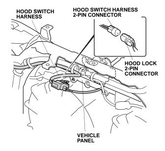
100. Remove the tape and plug the hood switch harness 2-pin connector into the engine starter harness 2-pin connector. Secure the connector to the vehicle harness with one wire tie.
