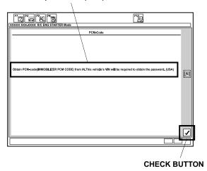
10. Input the PCM Code, then click the check button. NOTE: To ensure security, the PCM code (password) is changed every day, so it is impossible to register the remote controlled engine starter if the date of the PCM code acquisition and registration are different. The date of the HDS tester should also be the same.
