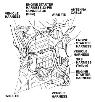
58. Secure the engine starter harness 23-pin connector (blue), and the engine starter harness to the vehicle harness with three wire ties.
