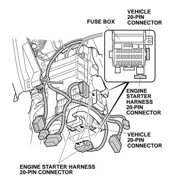
50. Unplug the vehicle 23-pin connector from the underside of the fuse box and plug the engine starter harness 23-pin connector (white) into the fuse box.
