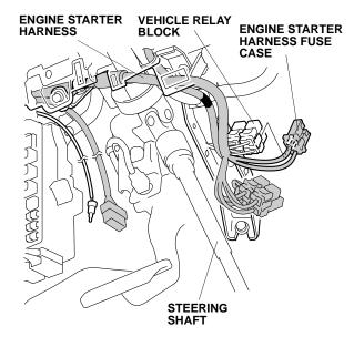
73. Align the white tape on the engine starter harness to the vehicle clip, and secure the engine starter harness to the vehicle harness with one wire tie.
