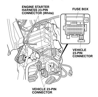
51. Unplug the vehicle 24-pin connector from the underside of the fuse box and plug it into the engine starter harness 24-pin connector as shown.
