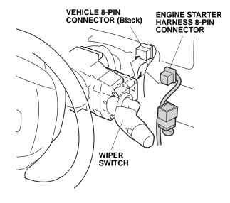
70. Plug the vehicle 8-pin connector (black) to the engine starter harness 8-pin connector.
