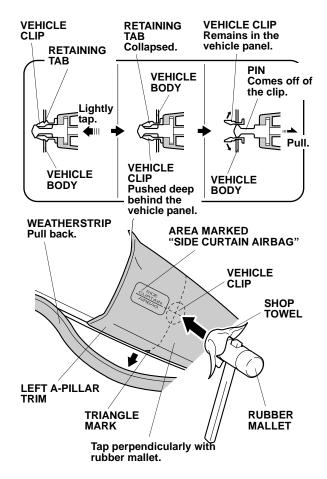
11. Using a rubber mallet wrapped with a shop towel, lightly tap the area marked "SIDE CURTAIN AIRBAG" on the top of the left A-pillar trim to push in the vehicle clip. Make sure to tap perpendicular to the A-pillar trim.
