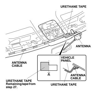
33. Using isopropyl alcohol on a shop towel, thoroughly clean the area where the urethane tape will attach. Secure the antenna cable to the vehicle panel with one urethane tape. Be careful not to crease the headliner.
