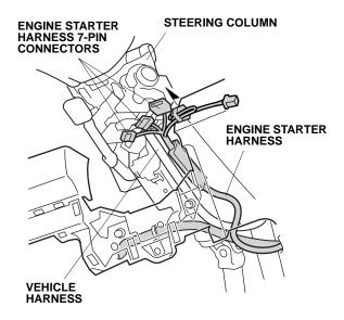
64. Unplug the vehicle 7-pin connector (brown) from the ignition switch and plug in the engine starter harness 7-pin connector (brown) as shown.
