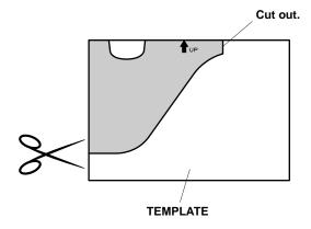
24. Align the template with the edge of the black ceramic paint, and secure it to the windshield with tape.
