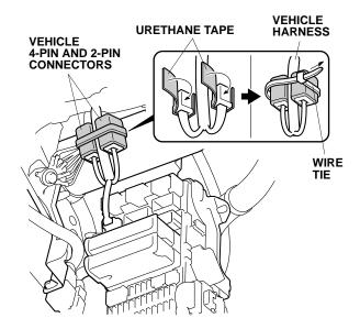
44. Secure the vehicle 4-pin connector and 2-pin connector to the vehicle harness using a wire tie.
