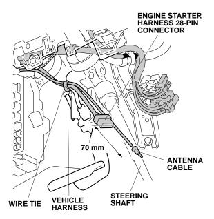
76. Secure the engine starter harness and antenna cable to the vehicle harness with one wire tie.
