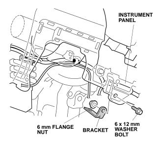
62. Attach the wire tie with clip to the engine starter harness at the white tape, then push the clip into the hole in the bracket.
