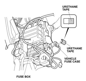
54. Wrap the vehicle fuse case with one urethane tape half cut in step 26.
