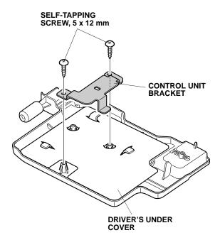
80. Install the control unit to the control unit bracket.
