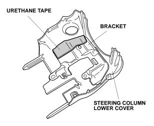
82. Attach a urethane tape to the bracket on the steering column lower cover.
