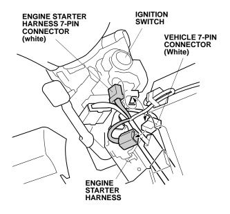
67. Place the vehicle 7-pin connector (brown) into the gap of the column.
