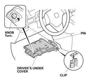
15. Remove the driver's lower cover (seven clips and two hooks).
