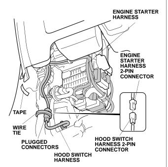
101. Plug the engine starter harness 28-pin connector and antenna cable into the control unit as shown.
