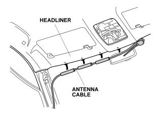
32. Using isopropyl alcohol on a shop towel, thoroughly clean the area where the urethane tape will attach. Cut the urethane tape remaining from step 27 as shown. Secure the antenna cable to the vehicle panel with the piece of urethane tape. Be careful not to crease the headliner.
