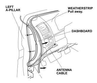
36. Route the antenna cable down under the dashboard. Tuck the antenna cable between the left A-pillar and the dashboard, then reinstall the weatherstrip.
