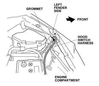
95. Route the hood switch harness. Secure the hood switch harness to the vehicle panel with the three clips installed on the hood switch harness.
