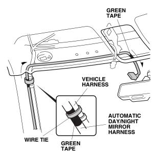
25. Route the automatic day/night mirror harness as shown. Secure the automatic day/night mirror harness to the vehicle harness at the green tape with one wire tie.
