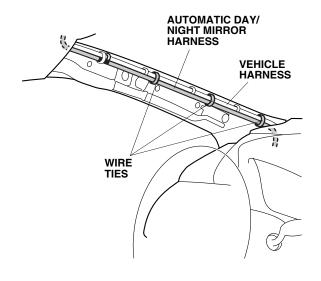
31. Secure the automatic day/night mirror harness to the vehicle harness using two wire ties in the areas shown.
