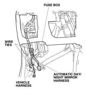
33. Attach the (2A) fuse label to the fuse case on the automatic day/night mirror harness.
