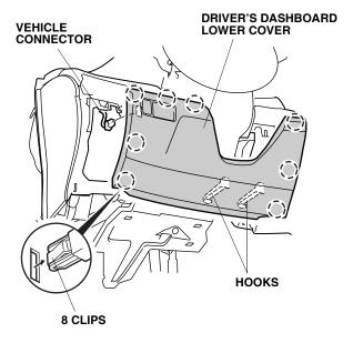
15. V6 only: Remove the driver's dashboard under cover (three clips and one pin).
