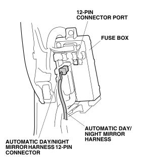
If another accessory connector is plugged into the 12-pin connector, remove the dummy connector from the other 12-pin connector harness and connect the automatic day/night mirror harness 12-pin connector into the other accessory harness.
