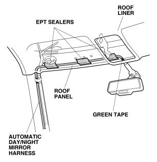
30. Secure the automatic day/night mirror harness to the vehicle harness using three additional wire ties.
