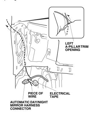
24. Remove the electrical tape and wire from the automatic day/night mirror harness.
