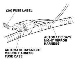
34. Plug the automatic day/night mirror harness 12-pin connector into the fuse box 12-pin connector port.
