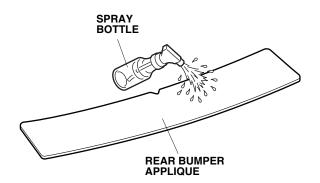
7. Align the V-notch in the rear bumper applique with the center of the trunk lid anchor as shown. Smooth the rear bumper applique along the rear bumper and tape each end at the curve in the bumper.
