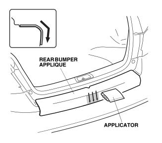
12. Use the applicator to apply the rear bumper applique to the rounded rear edge on the left side as shown. Start in the middle and work outward. Repeat on the right side.
