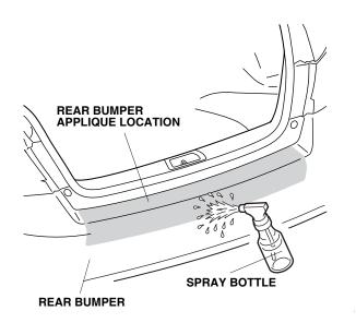
5. Remove the adhesive backing from the rear bumper applique.
