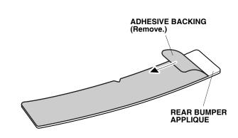
6. Using the spray bottle with 3M protective tape application solution, spray the rear bumper applique.
