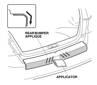
13. Remove the protective film from the rear bumper applique. Remove the protective film slowly; do not pull up the protective film.
