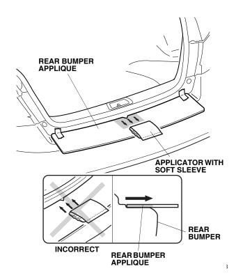
10. Starting at the center and working outward, use the applicator to smooth the rear bumper applique. Stroke in one direction only. Repeat on the right side.
