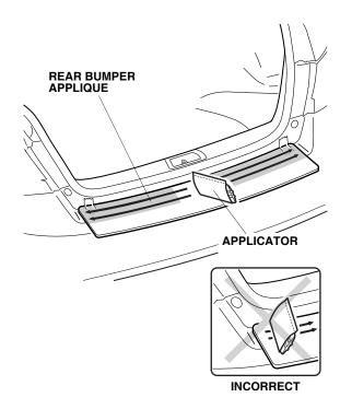
11. Once the upper surface is completely smooth with no bubbles, use the applicator to apply the rear bumper applique to the rounded rear edge at the center as shown.
