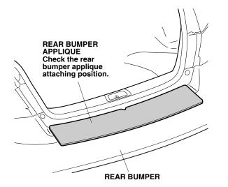
4. Using a spray bottle with 3M protective tape application solution, spray the rear bumper where the rear bumper applique will attach.
