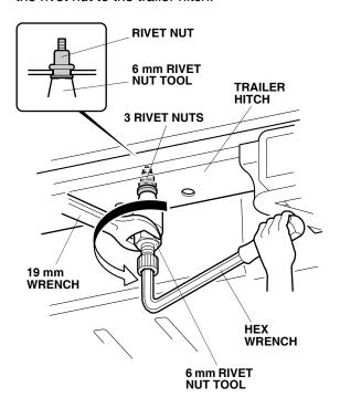
14. Remove the 6 mm rivet nut tool from the rivet nut by turning the hex wrench counterclockwise. Install two more rivet nuts in the holes in the trailer hitch.
