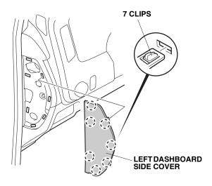
4. Remove the driver's dashboard lower cover (one self-tapping screw, nine clips, unplug one vehicle connector).
