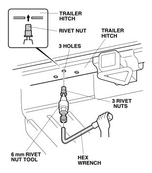
13. Holding the 6 mm rivet nut tool with the hex wrench, turn the 19 mm wrench counterclockwise and install the rivet nut to the trailer hitch.
