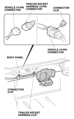
18. Install the connector clip into the vehicle 10-pin connector, and push the connector clip and trailer socket harness clip into the holes of the body panel.
