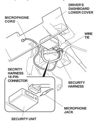
28. Fold the security harness and microphone wire, and secure it with one wire tie so that there is no tension applied to the microphone jack.
