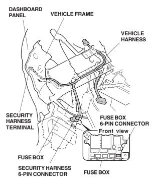
Route the security harness 2-pin connector along the vehicle harness, and route the security harness terminal between the vehicle frame and dashboard panel. 18. Remove the vehicle ground bolt, and attach the security harness ground terminal using this bolt.
