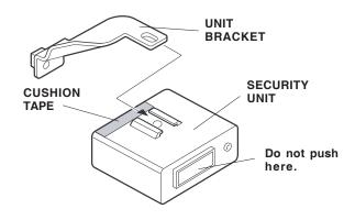
24. Insert the unit bracket into the security unit. Do not push at the connector area.
