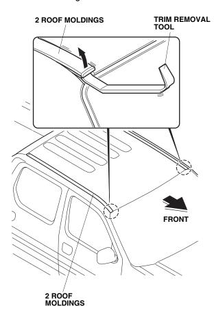
2. Slide and remove two roof moldings from the vehicle.
