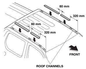
5. Reinstall the center and rear pieces of the roof molding to the roof channels.
