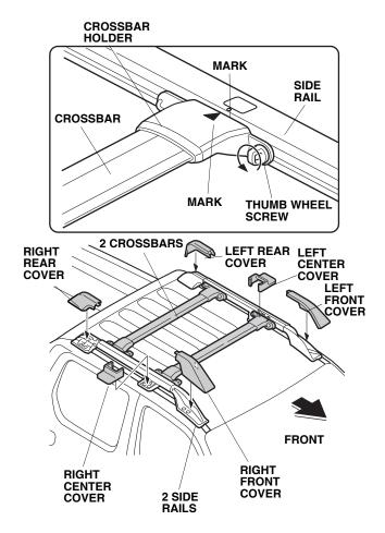
12. Loosen four thumb wheel screws on the crossbar holders. Align the marks on the crossbar holders with the marks on the side rails. Securely tighten the thumb wheel screws.
