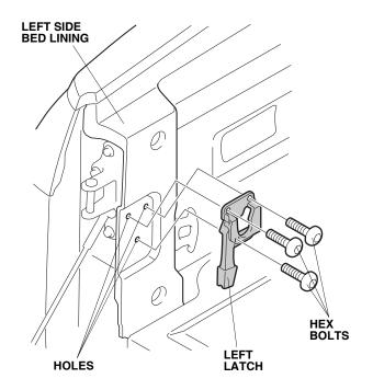
2. Install the left latch to the left side bed lining with three hex bolts.
