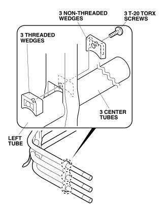
18. Insert three center tubes to the right tube (with label).
