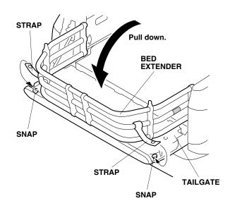
23. Secure two straps on the bed extender to two snaps on the tailgate.
