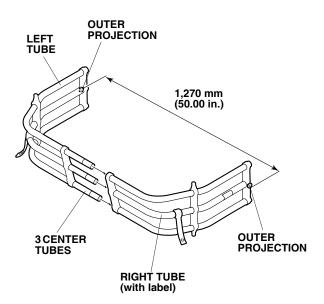
19. Adjust three center tubes so that the distance between the outer projections on the ends of the right tube (with label) and left tube is 1,270 mm (50.00 in.).
