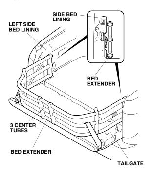
25. Align the non-threaded wedge with the threaded wedge at three joints between the right and center tubes, then secure the wedges with one T-20 torx screw each.
