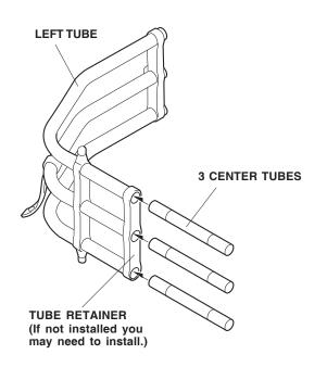
2. Align the non-threaded wedge with the threaded wedge at each of the three joints between the left and center tubes, then install one Torx screw through each pair.
