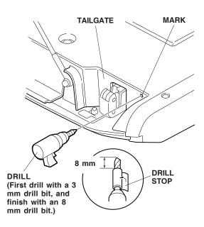
12. Press one fenderwell nut into the drilled hole in the tailgate.
