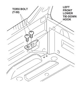
8. Install the left bracket and the left front lower tiedown hook using the two Torx bolts you removed.
