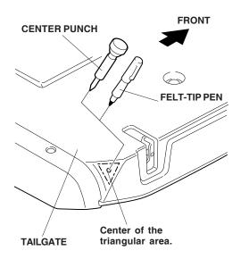
11. While wearing eye protection, drill an 8 mm hole through the center-punched mark on the left side of the tailgate. Use a drill stop to avoid drilling through the inner panel. First drill with a 3 mm drill bit, and finish with an 8 mm drill bit. After drilling, remove all burrs from the edges of the hole with a file.
