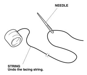
Starting in the back of the left spoke, lace the string through the holes of the steering wheel cover from the inside. Leave approx. 100 mm (3.93 in.) of string at the end. This will be used to tie the string at the end.
