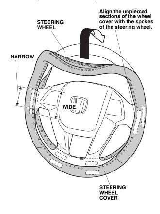
Turn over the steering wheel cover. Peel back the adhesive backings shown, and temporarily attach them to the front of the steering wheel cover with masking tape.
