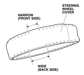
Place the wheel cover over the steering wheel with the unpierced sections of the wheel cover lined up with the spokes of the steering wheel as shown.
