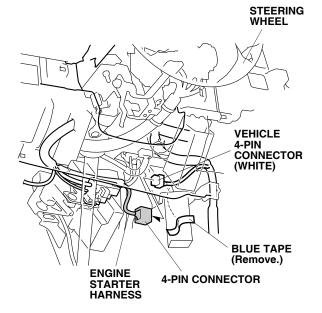
34. Secure the 4-pin connector to the vehicle harness with one wire tie.
