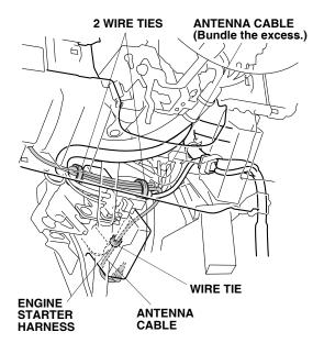
71. Bundle the excess antenna cable. Secure the antenna cable to the engine starter harness with two wire ties.
