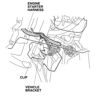
31. Route the engine starter harness relay block to the right side of the vehicle.
