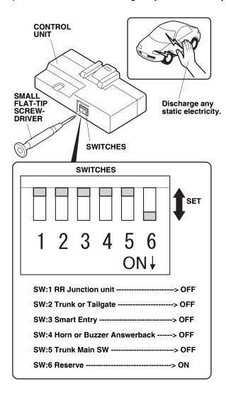
Check the location of the switches on the control unit.
