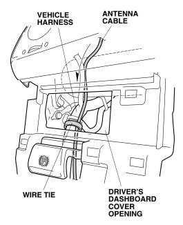
68. Route the antenna cable along the engine starter harness. Secure the antenna cable to the vehicle harness with the two wire ties that loosely secure the engine starter harness in step 44.
