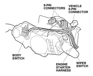
48. Route the engine starter harness into the harness case.
