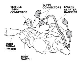
47. Unplug the vehicle 8-pin connector, and plug it into the engine starter harness 8-pin connectors. Plug the remaining engine starter harness 8-pin connector into the wiper switch.
