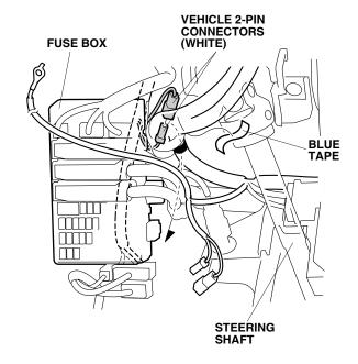
37. Plug the engine starter harness 2-pin connectors to the vehicle 2-pin connectors as shown.
