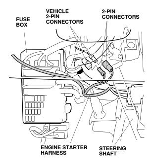
38. Route the engine starter harness 2-pin connectors behind the fuse box as shown.
