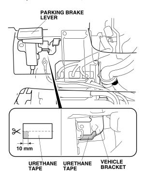
41. Clean the vehicle bracket surface where the urethane tape will attach with isopropyl alcohol. Attach the 10 mm piece of urethane tape that you cut in step 40 to the vehicle bracket as shown.
