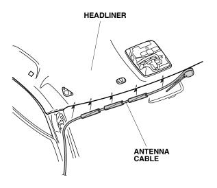
64. Clean the vehicle panel surface where the urethane tape will attach with isopropyl alcohol. Secure the antenna cable to the vehicle panel with one half of the urethane tape that you cut into two in step 40. Be careful not to crease the headliner.
