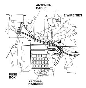
69. Route the antenna cable terminal to the right side of the vehicle, and plug it into the control unit as shown.
