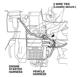
45. Route the engine starter harness 5-pin connector to the ignition switch.
