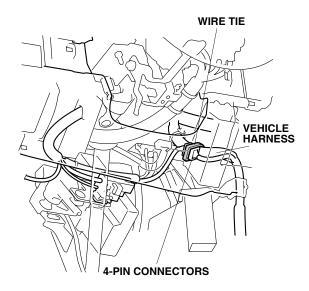
35. Align the green-taped part of the engine starter harness with the vehicle clip. Secure the engine starter harness to the vehicle harness with one wire tie.
