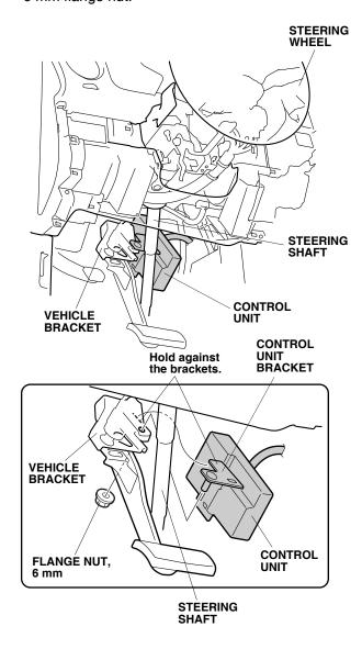
29. Install the engine starter harness fuse block clip on the control unit bracket.
