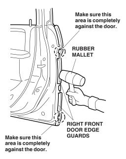
7. Repeat steps 3 thru 6 to install the left front door edge guards.
