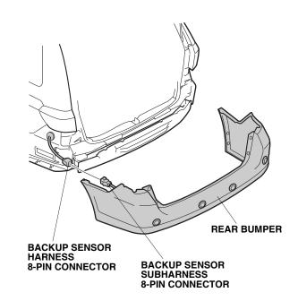
64. Install the rear bumper back onto the vehicle.
