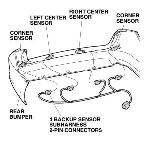
61. Secure the backup sensor subharness to the sensor clip at the green tape with four wire ties as shown.
