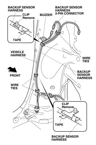
40. Secure the backup sensor harness to the vehicle panel with four wire ties.
