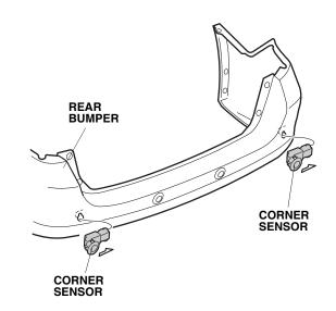
59. From the inside of the rear bumper, insert the two corner sensor clips to the two corner sensors.
