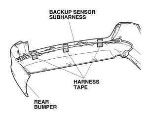
63. Bring the rear bumper to the vehicle and plug the backup sensor subharness 8-pin connector to the backup sensor harness 8-pin connector.
