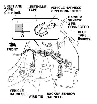
27. Cut a urethane tape in half and using that half, wrap the connector. Secure the connector to the vehicle harness with a wire tie. Go to step 34.
