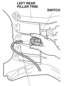
BACKUP SENSOR HARNESS 3-PIN CONNECTOR 51. For the left rear pillar trim, insert the clip matching the upper tab and install the trim. At the time of installation, take care that the switch does not come into contact with the left rear pillar trim.
