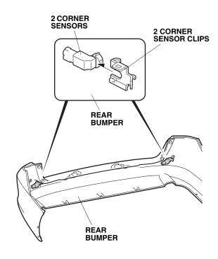
60. Plug the four backup sensor subharness 2-pin connectors to the right center sensor, left center sensor, and two corner sensors.
