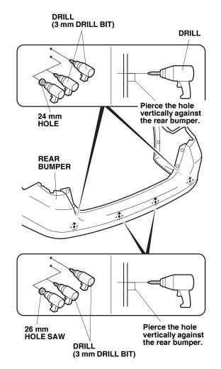
55. While wearing eye protection, drill 3 mm hole at the four pierced marks on the center of the rear bumper from the outside. Widen the two lower holes with 26 mm hole saw as shown. Remove any burrs.
