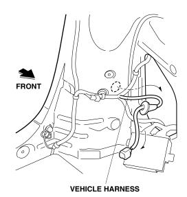
18. Bundle the vehicle harness as shown and secure it to the vehicle harness with one wire tie.
