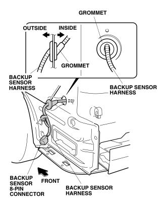
21. Remove the tape from the backup sensor harness. Plug the backup sensor harness 2-pin connector to the power tailgate sensor 2-pin connector.
