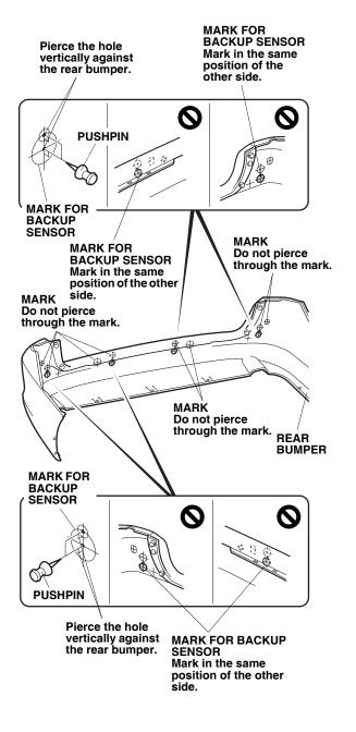
54. While wearing eye protection, drill 3 mm hole at the four pierced marks on the corner of the rear bumper from the outside. Widen the two lower holes with 24 mm hole saw as shown. Remove any burrs.
