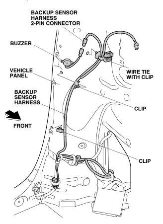
38. Install a wire tie with clip to the backup sensor harness and secure the clip to the vehicle panel.
