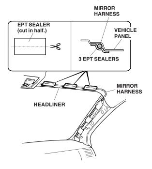
30. Route the ground terminal end from the mirror harness along the headliner and down the left A pillar towards the left fuse box.
