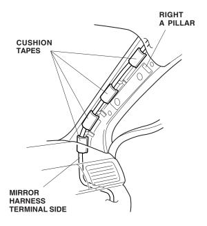
29. Using isopropyl alcohol on a shop towel, clean the headliner area where the mirror harness will attach. Using scissors, cut two EPT sealers in half. Using three halves of EPT sealers, attach the mirror harness to the vehicle panel.
