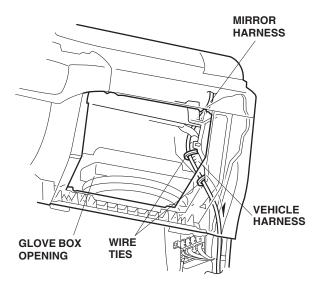
28. Using isopropyl alcohol on a shop towel, clean the right A pillar area where the mirror harness will attach. Attach the mirror harness to the right A pillar using four cushion tapes.
