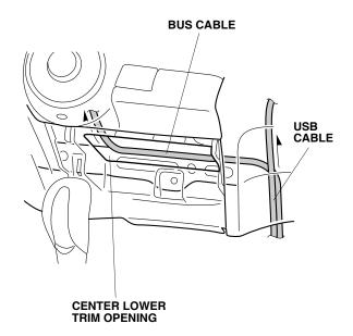
27. Align the bus cable 14-pin connector with the vehicle 24-pin connector, and secure the bus cable to the vehicle harness with one wire tie.
