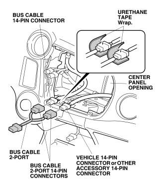
42. Plug the bus cable 14-pin connector or bus cable 2-port 14-pin connector into the audio unit, and reinstall the audio unit.
