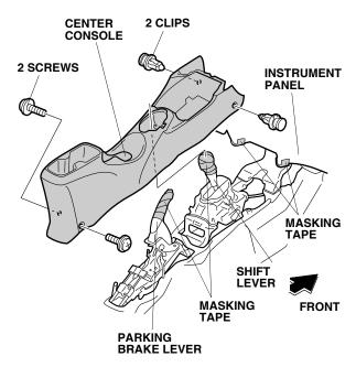
13. Carefully remove the center console (two clips and two screws).
