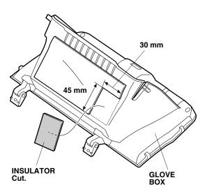
33. Using a pushpin, pierce the glove box in two places at the measurements shown.
