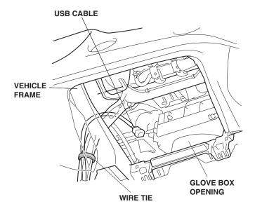
31. Secure the USB cable to the vehicle harness with one wire tie.
