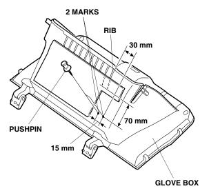
34. While wearing eye protection, drill the two pierced marks in the glove box. First drill with a 3 mm drill bit, and finish with a 16 mm hole saw. Use a utility knife to cut between the two 16 mm holes. Remove any burrs.
