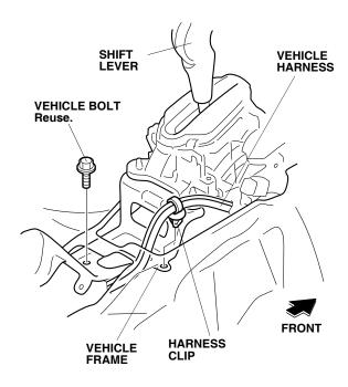
15. Position the control unit bracket under the floor carpet as shown.
