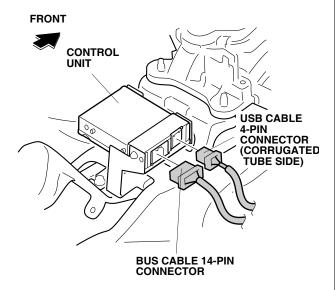
21. Route the bus cable and the USB cable forward along the vehicle harness.
