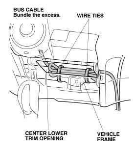
29. Route the USB cable into the glove box opening.
