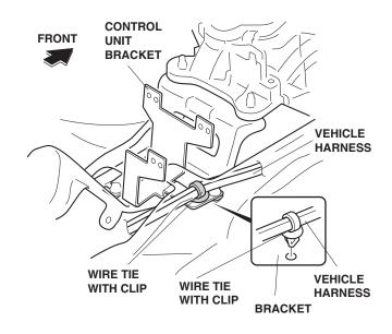
19. Install the control unit to the control unit bracket with three 5 x 7 mm flange bolts. Use a combination wrench to tighten three 5 x 7 mm flange bolts.
