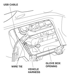
32. Get the glove box. Using a utility knife, cut out the insulator on the glove box at the measurement shown.
