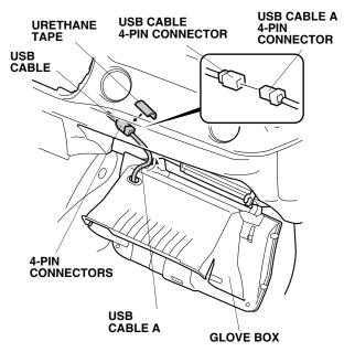
38. Wrap one urethane tape around the 4-pin connectors.
