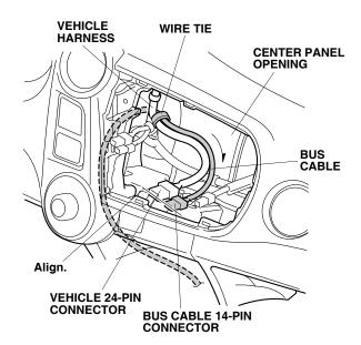
28. Bundle the excess bus cable, and secure it to the vehicle frame with two wire ties.
