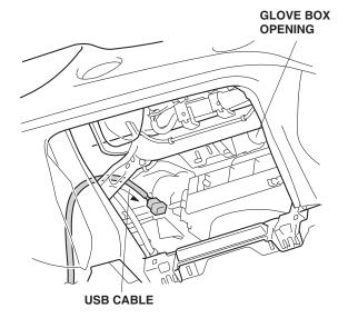
30. Secure the USB cable to the vehicle frame with one wire tie.
