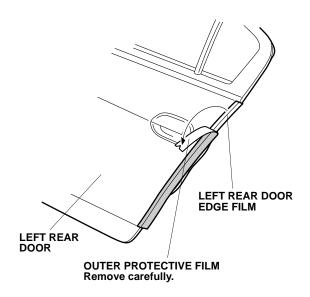
21. Starting from the center and working outward, fold the left rear door edge film around the left rear door edge. Move the applicator in only one direction. Be careful not to damage the door seal during this procedure.
