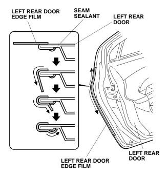
22. Using a shop towel, wipe the 3M protective tape application solution from the left rear door edge film. Allow the left rear door edge film to dry thoroughly.
