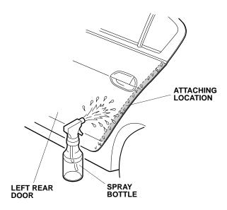
15. Using a spray bottle with 3M protective tape application solution, spray the area where the left rear door edge film will attach.
