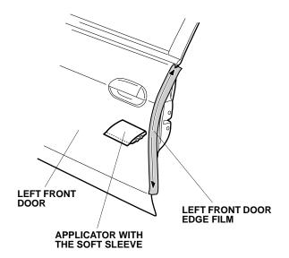
9. Carefully remove the outer protective film from the left front door edge film.
