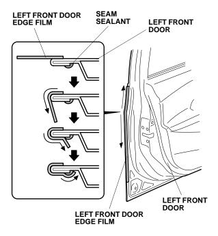
11. Using a shop towel, wipe the 3M protective tape application solution from the left front door edge film. Allow the left front door edge film to dry thoroughly.
