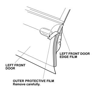
10. Starting from the center and working outward, fold the left front door edge film around the left front door edge. Move the applicator in only one direction. Be careful not to damage the door seal during this procedure.
