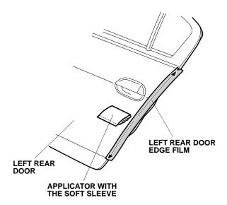
20. Carefully remove the outer protective film from the left rear door edge film.
