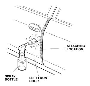
4. Using a spray bottle with 3M protective tape application solution, spray the area where the left front door edge film will attach.
