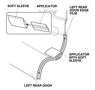
15. When you satisfied that the door edge film is firmly attached to the edge of the door, slowly remove the outer protective film.
