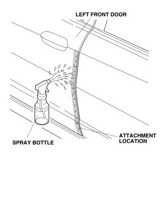
3. Open the left front door again. Peel back about 50 mm (2 in.) of adhesive backing from the left front door edge film. Align the V-notch in the door edge film with the end of the character line on the upper part of the front door.
