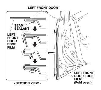
8. Using a lint-free shop towel, wipe up water from the front door edge film. Allow the front door edge film to dry thoroughly.
