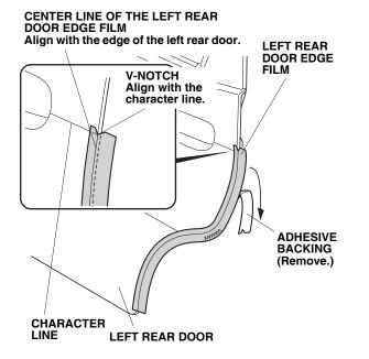
13. Continue to remove the adhesive backing while you align the center line on the door edge film with the edge of the door.
