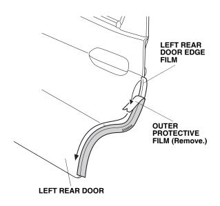
16. Starting in the middle of the door edge film and working outward, fold the door film around the door edge using your fingers. Move your fingers in one direction. Attach the film over the seam sealant. Do not trim or damage the seam sealant.
