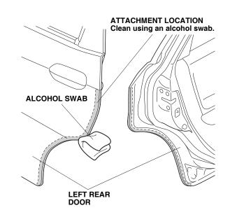
11. Close the left rear door. Using a spray bottle with 3M protective tape application solution, spray the area where the left rear door edge film will attach.
