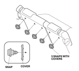
5. Install one clip to the inside of the tailgate frame on each side of the tailgate.
