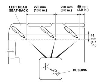
4. Insert the snaps through the covers, then install the snaps at the pierced marks.
