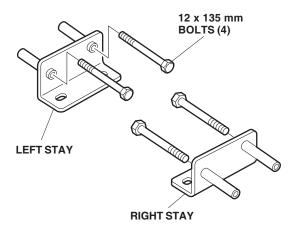
23. From the inboard side of the vehicle frame, slide the right and left stays into the right and left rear frame rails.
