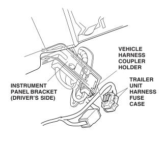
Connect the 12-pin connector of the trailer unit harness to the trailer unit.
