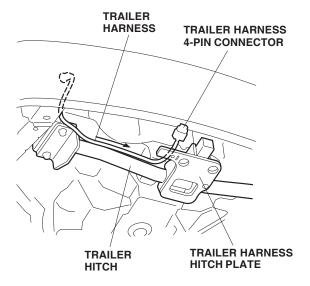
30. Install the connector bracket on the trailer harness 4-pin connector, and secure them to the trailer hitch with the flange bolt and flange nut. Route the trailer harness above the trailer hitch.
