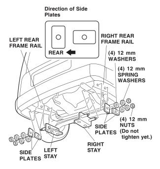
24. From the outboard side, slide the side plates onto the 12 x 135 mm bolts in the direction shown, then install the four 12 mm washers, four 12 mm spring washers and four 12 mm nuts on the ends of the 12 x 135 mm bolts. Do not tighten the nuts yet.
