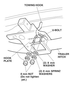
27. Torque all bolts and nuts to their specified torques in the order shown.
