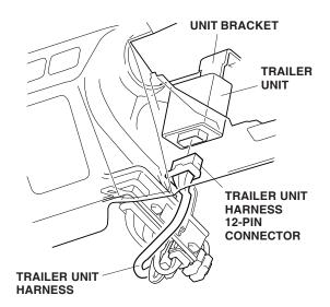
20. Secure the trailer unit harness with a wire tie to the instrument panel bracket.
