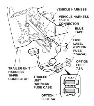
18. Install the trailer unit harness fuse case by sliding it onto the vehicle harness coupler holder.
