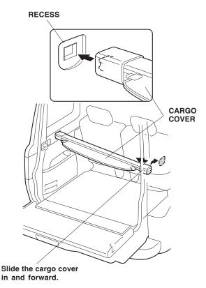
2. Install the cargo cover into the recess in the left rear side trim panel, then compress the cargo cover, and install it in the recess in the right rear side trim panel.
