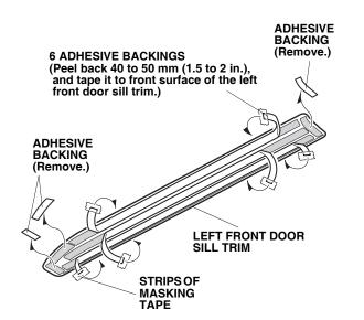
5. Starting at the curved area, push the left front door sill trim against the left front door sill. Align the edge of the left front door sill trim with the masking tape, and install the left front door sill trim.
