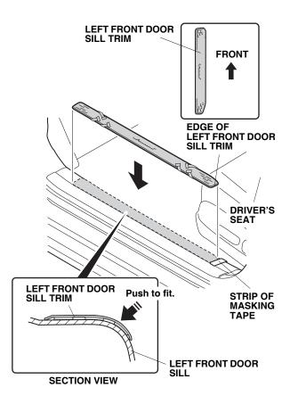
6. Using the palm of your hand, press on the left front door sill trim firmly against the door sill, and remove the adhesive backing in the order shown. Apply firm pressure especially at the ends.
