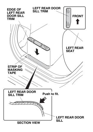
9. Using the palm of your hand, press on the left rear door sill trim firmly against the door sill, and remove the adhesive backings. Apply firm pressure especially at the ends.
