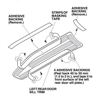
8. Starting at the curved area, push the left rear door sill trim against the left rear door sill. Align the edge of the left rear door sill trim with the masking tape, and install the left rear door sill trim.
