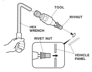
6. While holding the tool with the hex wrench, rotate the 27 mm wrench clockwise and install the rivet nut on the vehicle panel.
