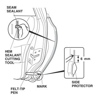
9. Position the hem sealant cutting tool against the door edge, and trim the seam sealant from mark to mark.
