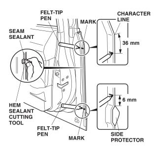
4. Position the hem sealant cutting tool against the door edge, and trim the seam sealant from mark to mark.
