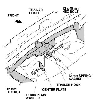
First torque the 10 x 40 mm bolts to 46 N·m (34 lb-ft), then torque the 12 x 45 mm bolts to 79 N·m (58 lb-ft).
