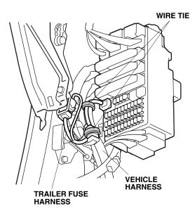
54. Insert the 5A fuse into the fuse box at the empty slot shown.
