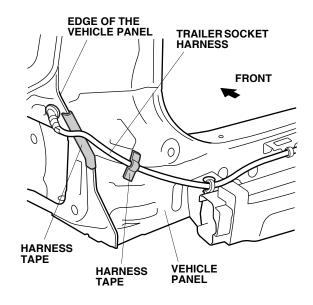
35. Inside the vehicle along the left cargo panel, locate the vehicle 8-pin connector blue-taped to the vehicle harness. Remove the blue tape to free the connector.
