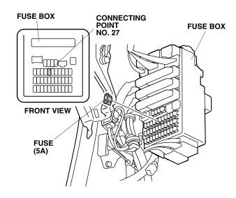
55. If an optional 5A fuse label is already attached to the driver's dashboard under cover, go to step 56. Otherwise, using an isopropyl alcohol on a shop towel, thoroughly clean the area where the fuse label will attach. Attach the 5A fuse label to the NO. 27 slot on the driver's dsshboard undercover.
