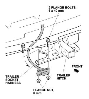
33. Secure the trailer socket harness to the trailer hitch at the green tape using one wire tie.
