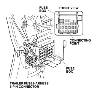
51. If another accessory connector is already plugged into the fuse box 6-pin connector, remove the dummy connector from the other accessory harness. Plug the trailer fuse harness 6-pin connector into the other accessory harness 6-pin connector.
