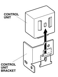
41. Plug the control unit harness 12-pin connector into the control unit, then secure the control unit harness to the control unit bracket using the wire tie with clip installed in 39.
