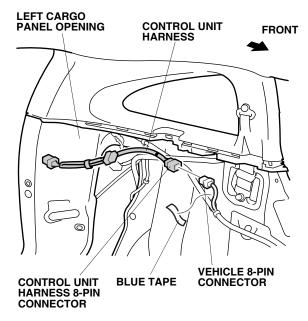
36. Get the control unit harness. Plug the control unit harness 8-pin connector into the vehicle 8-pin connector you just freed.
