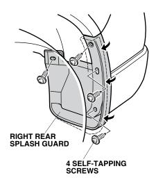
4. Remove the right splash guard (four screws and slide forward).
