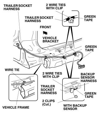
31. Secure the trailer socket harness to the vehicle frame with one additional wire tie.
