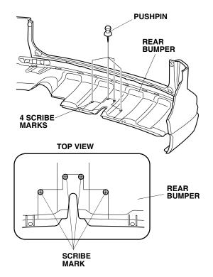
26. While wearing an eye protection, drill the rear bumper at each pierced mark using a 20 mm hole saw.
