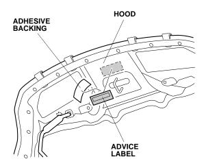
19. Remove the adhesive backing from the advice label and attach it to the hood as shown.
