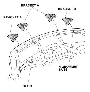
3. Close the hood. Attach pieces of masking tape to the hood under two brackets A and two brackets B as shown.
