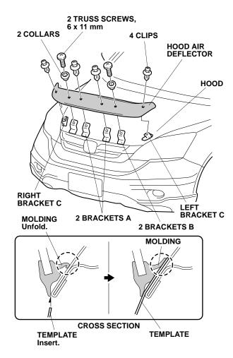
17. Using the large end of a template, insert it between the hood and hood air deflector to unfold the molding as shown.
