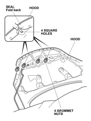
2. Align two brackets A and two brackets B to the holes on the four grommet nuts.
