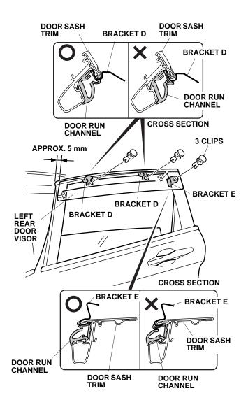
9. Using the palm of your hand, press down on the left rear door visor while removing the two adhesive backings. Make sure there is no clearance between the bracket and door sash trim.
