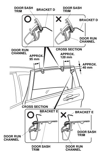
3. Position the left rear door visor on the door sash trim. Adjust the positions of the two brackets D and bracket E, and temporarily install the door visor with the three clips.
