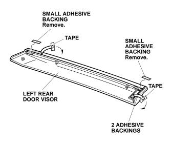
7. Remove the masking tape you attached in step 4.
