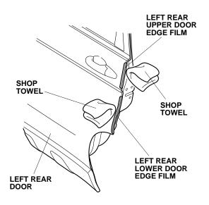
21. Repeat steps 1 through 20 to install the door edge film on the right side of the vehicle.
