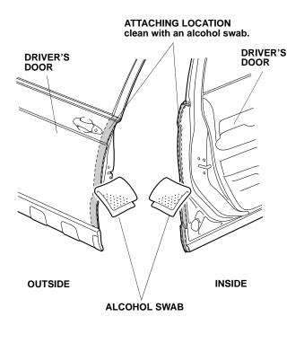
2. Close the driver's door. Using a spray bottle with 3M protective tape application solution, spray the area where the left front door edge film will attach.
