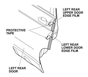
19. Starting from the center and working outward, use the applicator with the soft sleeve to fold the left rear upper door edge film and left rear lower door edge film inside the left rear door as shown. Move in one direction only. Do not damage the door seal during this procedure.
