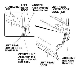
16. Align the center line on the left rear lower door edge film with the edge of the left rear door. While applying light pressure, carefully remove the adhesive backing, and attach the left rear upper door edge film to the left rear door.
