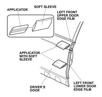
8. Slowly remove the protective tape from the left front upper door edge film and left front lower door edge film.
