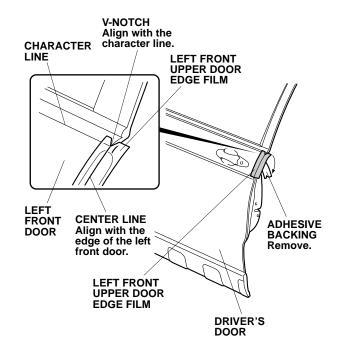
4. Align the center line on the left front upper door edge film with the edge of the left front door. While applying light pressure, carefully remove the adhesive backing and attach the left front upper door edge film to the driver's door.
