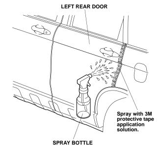
Open the left rear door. Peel back about 50 mm (2 in.) of adhesive backing from the left rear upper door edge film. Align the V-notch with the end of the character line on the upper part of the left rear door as shown.
