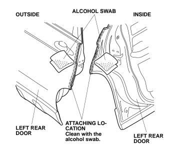
12. Using a spray bottle with 3M protective tape application solution, spray the area where the left rear door edge films will attach.
