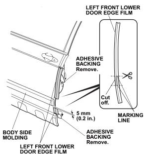
6. Align the center line on the left front door edge film with the edge of the left front door. While applying light pressure, carefully remove the adhesive backing and attach the left front lower door edge film to the driver's door.
