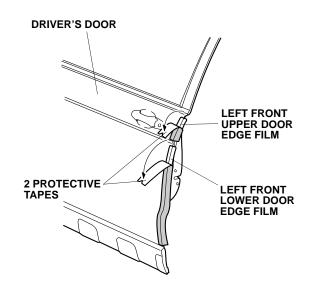
9. Starting from the center and working outward, use the applicator with the soft sleeve to fold the left front upper door edge film and left front lower door edge film inside the driver's door as shown. Move in one direction only. Do not damage the door seal during this procedure.
