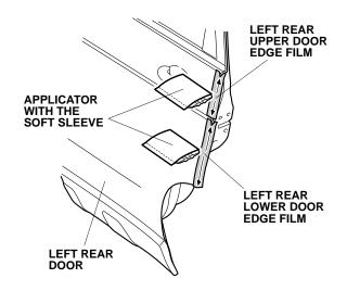
18. Slowly remove the protective film from the left rear upper door edge film, and left rear lower door edge film.
