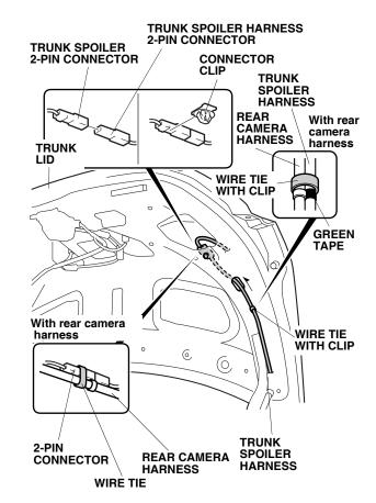
26. Install the connector clip to the 2-pin connector, and secure the 2-pin connector to the vehicle panel.
