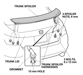
Fit the trunk spoiler into position on the trunk lid, and install the four 6 mm spoiler nuts and two 6 x 12 mm bolts. Hold the trunk spoiler firmly against the trunk lid and torque the spoiler nuts and bolts to 9 N·m (6.5 lb-ft).
