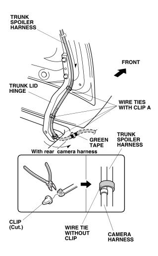
29. Route the trunk spoiler harness, and secure it to the vehicle panel holes with two wire ties with clip.
