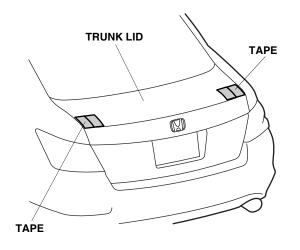
7. Close the trunk lid. Align the template with the edge of the trunk lid on the left side. Using a felt-tip pen, mark the trunk lid as shown on the template. Remove the template.
