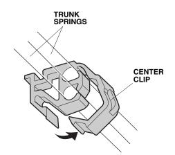
17. With an assistant holding the trunk lid open, remove the old trunk springs from the trunk hinge arms using the trunk spring tool. Wear gloves to protect your hands, and pull the trunk spring tool slowly and carefully towards you.
