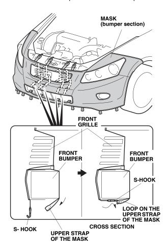
15. Attach the four plastic hooks to the bottom edge of the front bumper.
