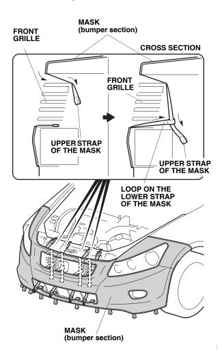
14. Continue routing the upper strap of the mask through the inside of the front bumper and attach the S-hook to the loop on the upper strap of the mask as shown. Repeat on the other straps.
