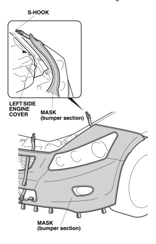
12. Attach two S-hooks to the bottom edge of the radiator cover.
