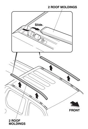
3. Using long nose pliers, remove six clips from the roof channels. Discard the clips.
