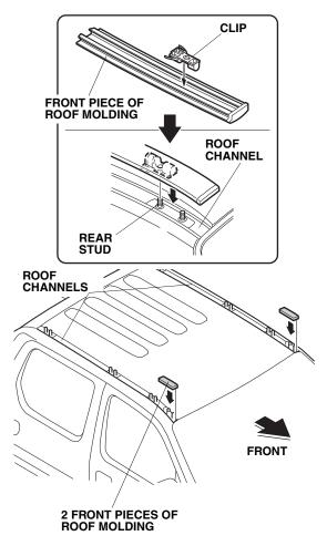
7. Reinstall the front pieces of the roof molding to the roof channels.
