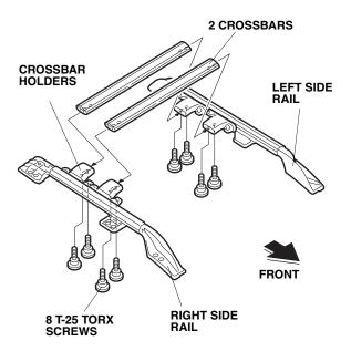
9. Align the holes on the left and right side rails with 12 studs in the roof channel. Adjust the position of the roof moldings installed in step 5 if necessary.
