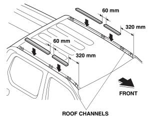
5. Reinstall the center and rear pieces of the roof molding to the roof channels.
