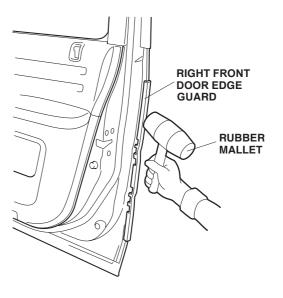
7. Repeat steps 3 through 6 to install the left front door edge guard.
