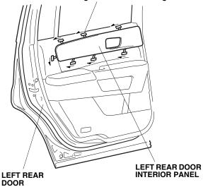
41. Using a rubber roller, apply pressure against the left rear door interior panel and roll from one end to the other.
