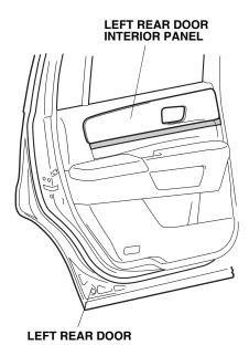
36. Using isopropyl alcohol on a shop towel, clean the area where the left rear door interior panel will attach.
