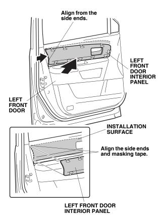
24. Press the left front door interior panel firmly to attach while removing the adhesive backings that you temporarily attached to the surface side.
