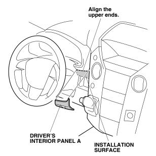
11. Press the driver's interior panel A firmly to attach while removing the adhesive backing that you temporarily attached to the surface side.
