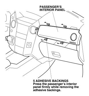
6. Using a rubber roller, apply pressure against the passenger's interior panel and roll from one end to the other.
