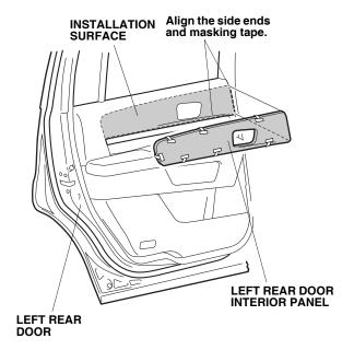
40. Press the left rear door interior panel firmly to attach while removing the adhesive backings that you temporarily attached to the surface side.
