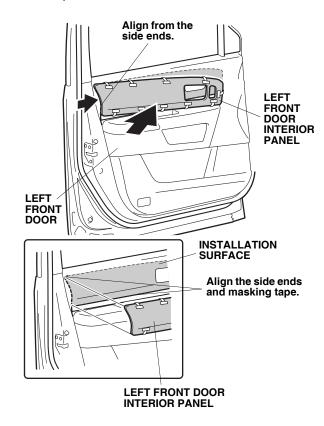
32. Press the left front door interior panel firmly to attach while removing the adhesive backings that you temporarily attached to the surface side.
