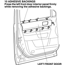
25. Using a rubber roller, apply pressure against the left front door interior panel and roll from one end to the other.
