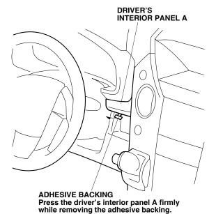
12. Using a rubber roller, apply pressure against the driver's interior panel A and roll from one end to the other.
