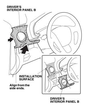
17. Press the driver's interior panel B firmly to attach while removing the adhesive backings that you temporarily attached to the surface side.
