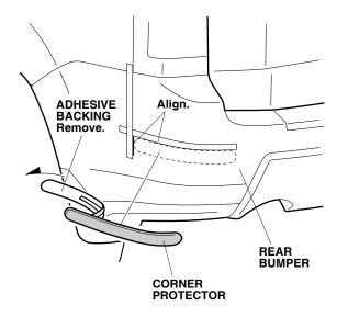
16. Attach the corner protector to the rear bumper by aligning it with the masking tapes.
