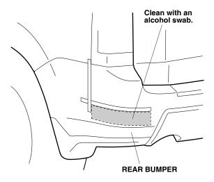
15. Remove the adhesive backing from the corner protector. Check the back of the corner protector for the correct orientation.
