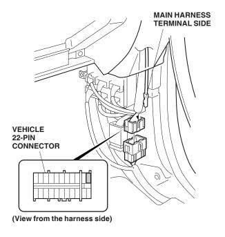
27. Secure the mirror harness to the vehicle harness using two wire ties.
