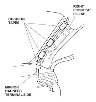
29. Using isopropyl alcohol on a shop towel, clean the headliner area where the mirror harness will attach. Using scissors, cut two EPT sealers in half. Using three halves of EPT sealers, attach the mirror harness to the vehicle panel.
