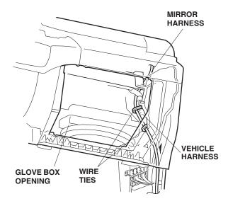
28. Using isopropyl alcohol on a shop towel, clean the right front "A" pillar area where the mirror harness will attach. Attach the mirror harness to the right front "A" pillar using four cushion tapes.
