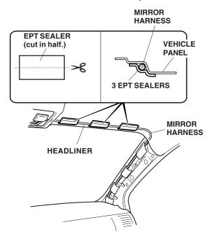
30. Route the ground terminal end from the mirror harness along the headliner and down the left front "A" pillar towards the left fuse box.
