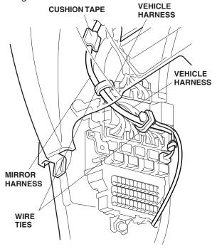
34. Using isopropyl alcohol on a shop towel, clean the vehicle panel. Attach the mirror harness to the vehicle panel using one cushion tape.
