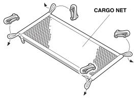
2. Position the cargo net with the zipper facing the rear of the vehicle. Attach the four cargo net hooks to the four tie-down rings.
