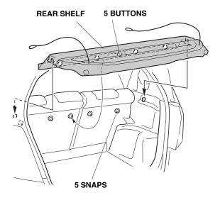
7. Hook the cord on each side of the rear shelf to each clip installed on the tailgate.
