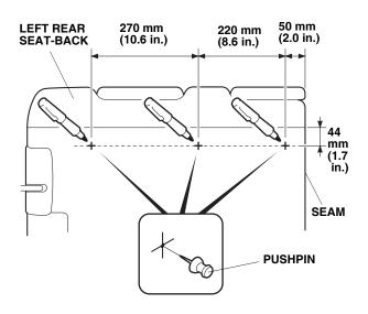
4. Insert the snaps through the covers and install the snaps at the pierced marks. Be careful not to overtighten the screws.
