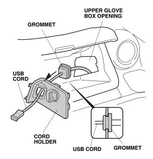
Install the cord holder into the upper glove box in place of the side cover and insert the end of the USB cord into the cord holder.
