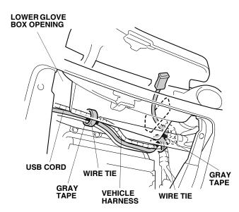
17. Using two wire ties, secure the USB cord to the vehicle harness in the areas shown.
