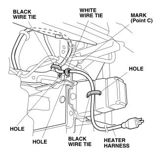
18. On SC Model; Cut off the rib shown, and trim the lower grille as necessary until the heater harness end fits through rhe opening.
