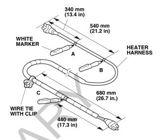
10. Plug the heater harness connector into the engine block heater, and route the heater harness over the engine. Secure the heater harness to the vehicle harness with one white wire tie in the area shown.
