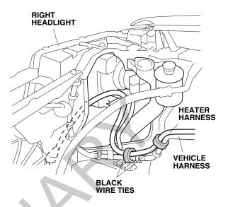
15. Route the heater harness along the vehicle harness and attach the wire tie with clip to the vehicle panel hole.
