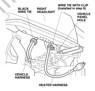
16. Using one black wire tie, secure the heater harness to the vehicle harness.
