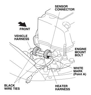
13. Continue routing the heater harness under the ABS unit bracket along the vehicle harness, and secure the heater harness to the vehicle harness with two black wire ties in the areas shown.
